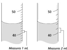
(*Hints*: Always check the unnumbered marks on a graduated cylinder to see what each mark indicates. Sometimes, the bottom of the meniscus falls between two markings. In that case, you need to estimate the measurement between the two marks.) Both of the graduated cylinders on the right contain the same volume of liquid. Although the cylinders have different markings, both cylinders contain 45 mL of liquid.
