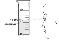
The graduated cylinder is a tool frequently used to measure liquid volume. ("Graduated" means that the cylinder is marked with measurement units.) Water in a graduated cylinder has a curved surface, as shown top right. The curved surface is called a meniscus. The volume should be read at the lowest point of the meniscus. Be sure to read the volume at eye level.
